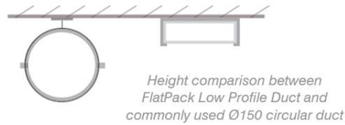
Today's architects and builders strive to achieve living and work spaces that make the most of a building's interior while being more cost effective and energy efficient. In order to achieve this, building designers are minimising the inner ceiling space and therefore reducing the space for installers to run the building's services.
